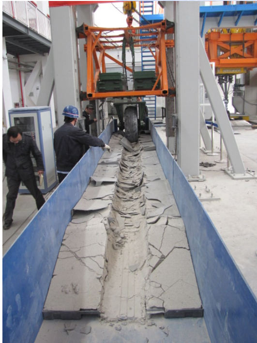
Fig. Equivalent single wheel load verification tests
